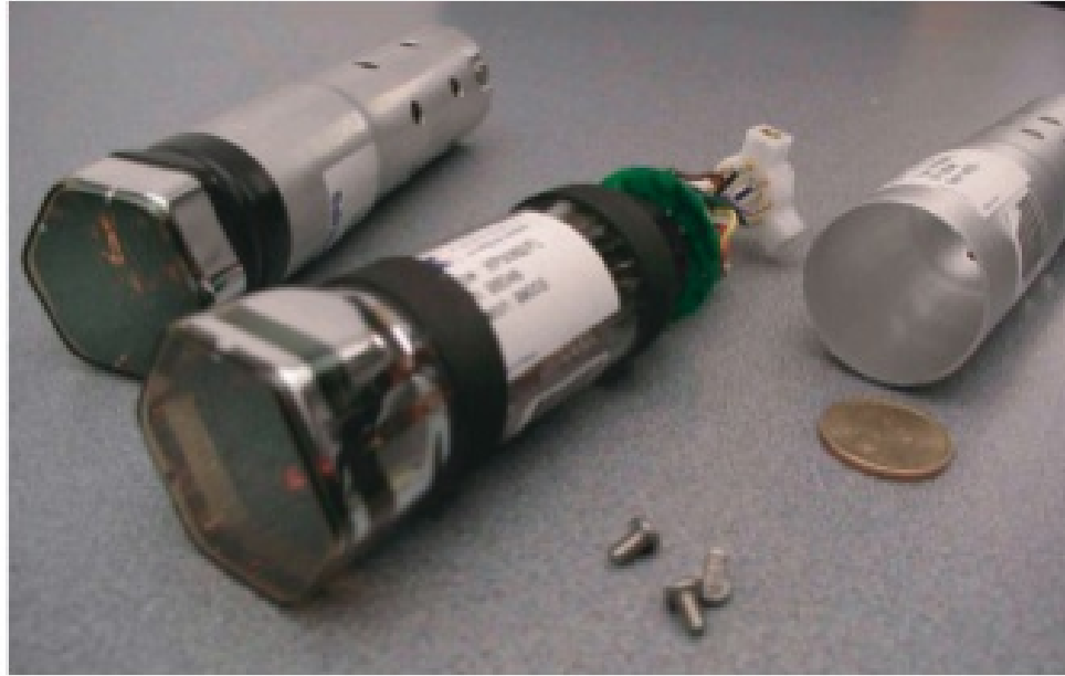
Figure 4.10. Photo multiplier tubes used in HiRes Experiment
