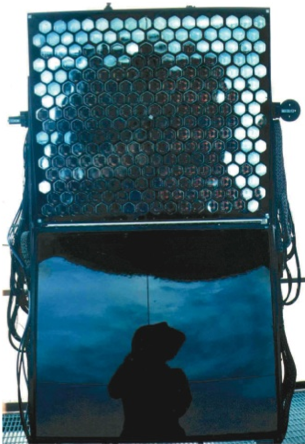
Figure 4.8. UV camera of HiRes detector - a cluster of PMTs
