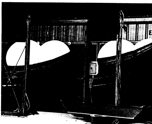
FIGURE 5. MIRROR UNITS for HiRes, the High Resolution Fly's Eye Detector. Each of the facility's 64 spherical-mirror units will comprise four glass segments and a cluster box (seen here from behind) in the focal plane, containing a mosaic of 256 hexagonal photomultiplier tubes. Two such units will be enclosed in each of 32 garage-type sheds arrayed over the project's two sites. Some of this may change in March, when a revised Auger proposal is expected in response to a review just completed by a subcommittee of DOE's High Energy Physics Advisory Panel.
