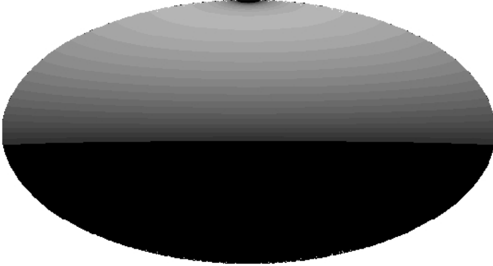
Fig. 11. AGASA estimated relative exposure, \rho_A(\delta) , for events above 10^{19.5} eV in equatorial coordinates (right ascension right to left). The lightest region corresponds to a normalized event density of \sim 1.6 . The observable sky extends from \delta = -8^\circ to \delta = 87.5^\circ .
