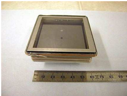
Figure 6: The BURLE 85001 Planacon TM multichannel plate photomultiplier.
