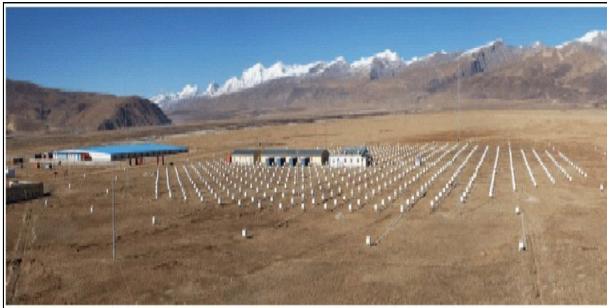
Figure 8. A photograph of the Tibet array at an altitude of 4300 m. The white objects is scintillation counter array with the central station containing the hadron detectors, which are burst and emulsion chamber units.
